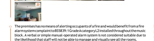
WHY The music block is a detached building away from the main block and is a single-storey building with multiple classrooms. Within the music block, there is no automatic fire detection system installed. A simple manual operating bell is installed within the entrance area of the music block. Although it was discussed that staff are present within the building at all times, there are serval rooms where a fire could start and be undetected for several minutes. LOCATION Music block HIGH
